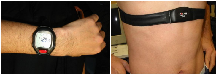
Fig. 4. The heart rate monitor. It can sense the heart rate via a small chest sensor worn around the chest and send the data using wireless technology to the watch. The watch terminal can record continuous heart rate during the workout.
