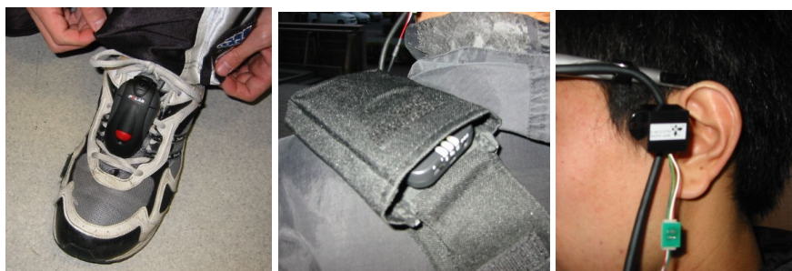
Fig. 5. The left image is a speed sensor which measures the accurate running speed/pace and distance. This sensor sends the data via wireless communication to the watch terminal as shown in Fig. 4. The center image is a GPS sensor device. This device can sense geographical location coordinate values sent to the PDA. The right image is a 3D motion sensor sensing motion data (x, y and z directions) that are also sent to the PDA.
